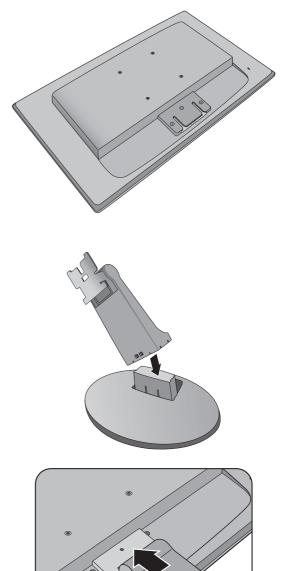
Orient and align the stand arm with the monitor, then push them together until they click and lock into place.
